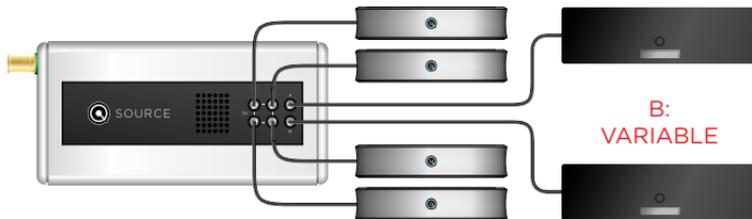
Once voltages are selected, connect all devices using their corresponding QSOURCE DC Cables (sold separately). Make sure to align the keys (indicated with red dots) on both the LEMO connector and the outputs before connecting them.
