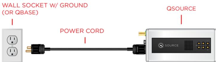
Once the correct VAC is selected and the device is plugged in, you may turn on the QSOURCE using the power switch located on the end of the unit, between the binding post and IEC input. **However, make sure the device is powered off while connecting devices or changing voltages.** A blue LED light will remain lit on the opposite end of the QSOURCE while it is active
