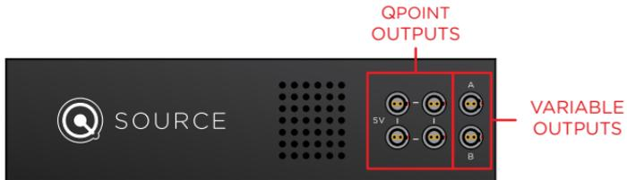
Outputs “A” and “B” are controlled by the corresponding switches on the bottom of the QSOURCE. Output “A” supplies 9, 19, or 12 VDC, while output “B” supplies 19, 24, or 12 VDC. Select the correct voltage necessary for your device before connecting any devices or powering on the QSOURCE.
